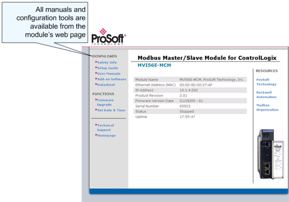
**Important:** The temporary IP address is only valid until the next time the module is initialized. Please refer to the *MVI56E-MCM User Manual* for information on how to set the module's permanent IP address.
