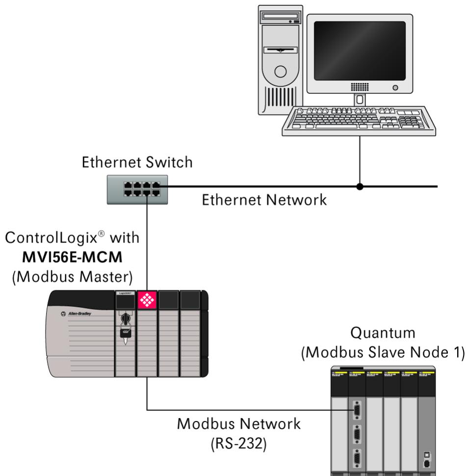
Note: The illustration does not show the required Ethernet connection for processor programming.
